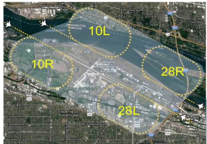
Runway numbers refer to compass bearing based on aircraft direction. A runway numbering of 28 refers to a direction of 280 degrees. 28L refers to the left of 2 runways both at 280 degrees.
